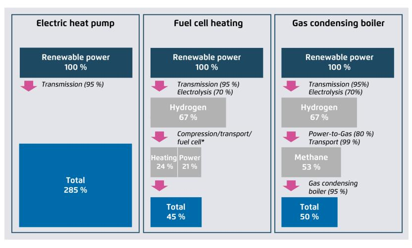
→ Boilers with renewable hydrogen (instead of fuel cells) yield a total efficiency of about 50 to 60 %.
