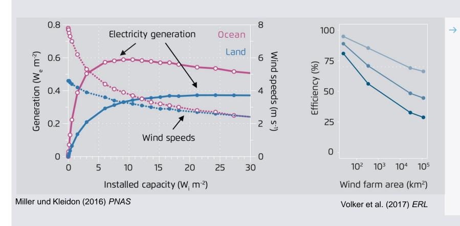
Climate model simulations show that many turbines reduce wind speeds, turbine efficiencies, and wind energy resource potentials
