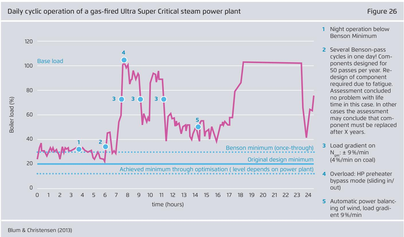
ity prices (e.g. due to high wind penetration), while avoiding a complete shutdown of the plant and continuing heat generation. Steam bypass systems can be installed relatively inexpensively (approximately 0.1 million DKK per MW, i.e. 0.01 euros per MW).<sup>27</sup>
