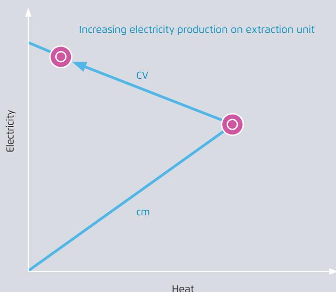
\* The  $C_b$  coefficient (back-pressure coefficient) is defined as the maximum power generating capacity in back-pressure mode divided by the maximum heat capacity. The  $C_v$  value for an extraction steam turbine is defined as the loss of electricity production when the heat production is increased by one unit at constant fuel input.
