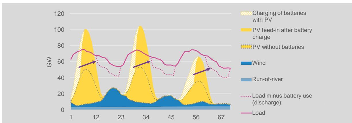
Source: Authors' assessment of Agorameter data for 21 – 23 May, 2014, scaled to 72 GW wind and 150 GW PV (70 GW PV without battery storage; 80 GW PV with 40 GW of battery output and 120 GWh of storage capacity)
