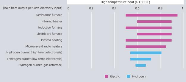
Agora Energiewende & AFRY (2021) Note: "Values" refer to lower heating values. The hydrogen burner efficiency is 90%. Efficiencies do not consider midstream losses. Hydrogen produced by gas reforming has gas as its energy input.
