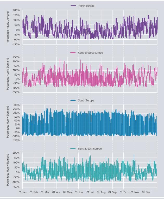
AFRY analysis. Units indicate the % of daily annual average hydrogen demand. That is, -100% means there is no hydrogen production for that period; 0% means that production and demand are balanced for that period; +100% means that production is twice as large as demand for that period.
