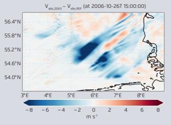
An example where the winds are from the southwest. The colour scale gives the wind speed difference in m/s. The lower wind speeds in the wind farms and surrounding areas mainly downwind of the wind farms and wind farm clusters, can be seen. Higher winds than those in the reference simulation can also be seen.
