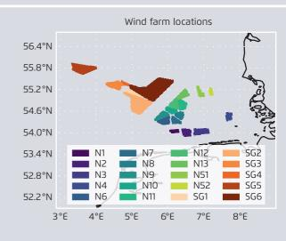
These two representations of wind farms are used in the mesoscale simulations and in the reference simulation without any wind farms. Each plotted coloured point represents a mesoscale grid box in which wind turbines are present.
